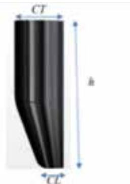
Figure 8. Basic Hydrofoil Dimension.
