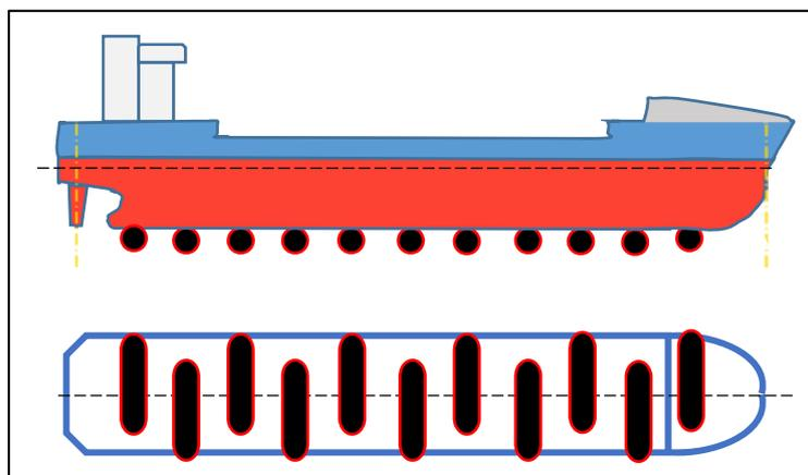
Figure 2. Staggered arrangement.
