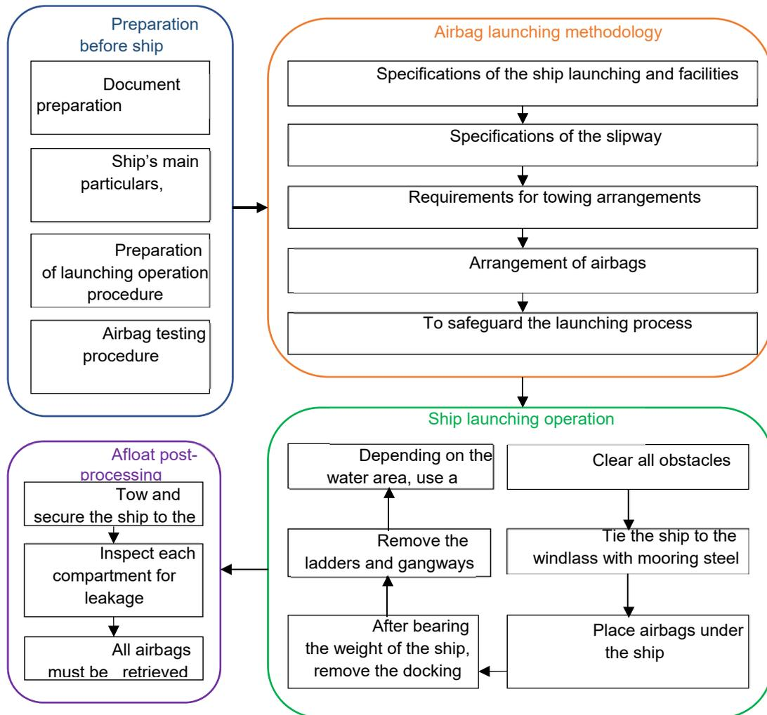
Figure 5. Ship launching operation flow.
