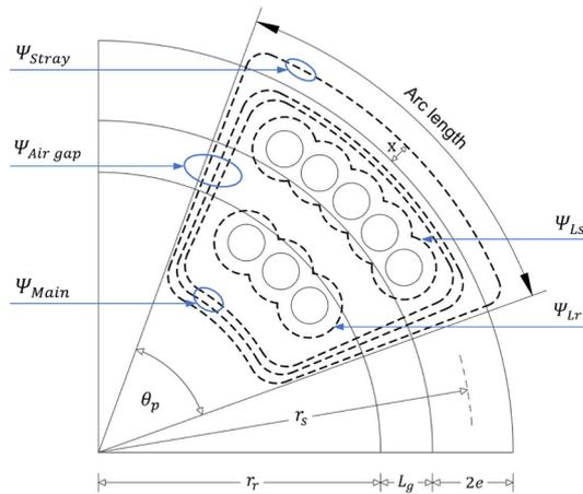
Figure 3. Illustration of stray flux; (Source: Koroglu *et al.*, 2009).
