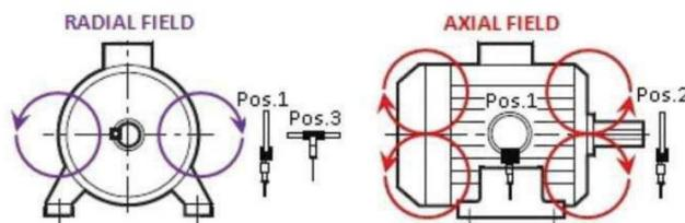
Figure 4. Coil sensor in different measurement positions; (Source: Ceban *et al.*, 2012).
