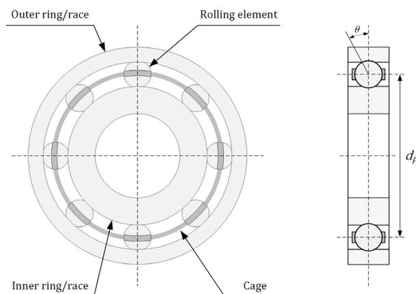
Figure 1. Bearing construction elements and cross section view; (Source: Authors).
