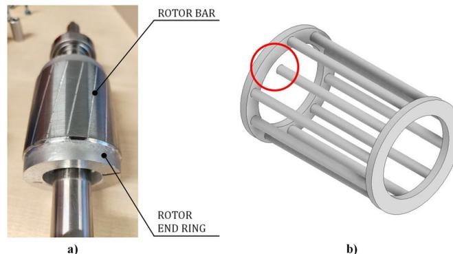
Figure 2. (a) Induction motor squirrel cage rotor; (b) Illustrative example of broken rotor bar; (Source: Authors).
