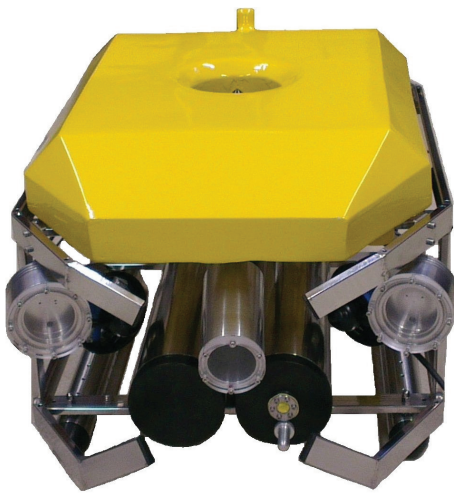
Figure 10. ROV frame, buoyancy block and vessels.
