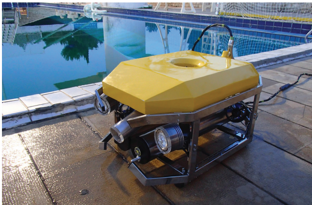
Figure 11. ROV during wet testing at the University swimming pool.
