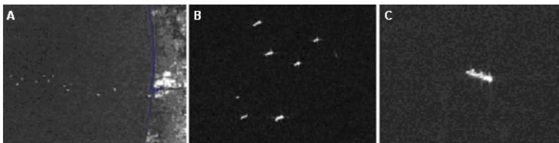
Figure 20. SSAR 50, 25 and 8 m Resolutions of Ships Images – Source: İlcev (2016).
